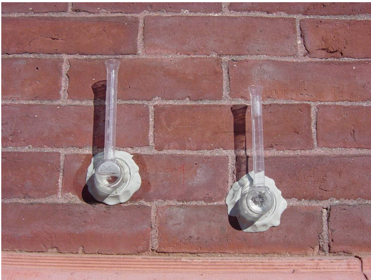
Photo 29 - RILEM test 11.4. This test is used to measure the absorptivity of the brick and mortar. At the test on the left above, the brick rapidly absorbed the water and failed in 30 seconds. The test of the mortar on the right failed in 19 minutes. The more rapid the failure, the more absorptive the material. See the body of the report for more information on the test.
